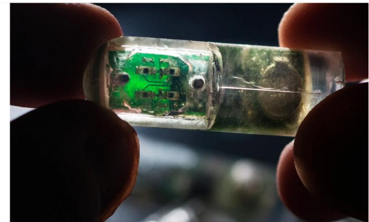
MIT researchers built an ingestible sensor equipped with genetically engineered bacteria that can diagnose bleeding in the stomach, possibly other gastrointestinal ailments. LILLIE PAQUETTE/MIT
